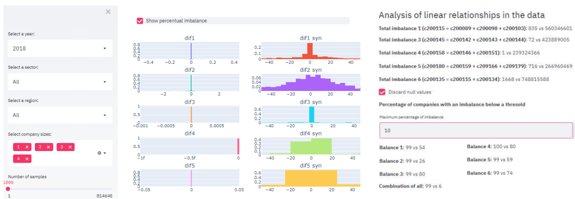
Figure 10 Comparison between the percentual imbalance of five linear balance equations, computed from real (left histograms) and synthetic (right histograms) data.
